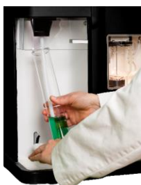
Fig. 1. Inserting a tube in the KjelROC Analyzer
